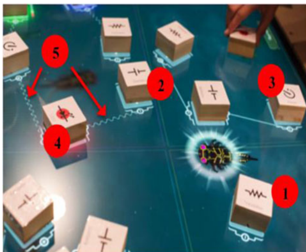
Fig. 2 Players assemble virtual circuits using wooden blocks that represent resistors (1), batteries (2), timers (3), and different colored LEDs (4). Participants make circuit connections (depicted as lines on the tabletop (5) by bringing the positive and negative terminals of the blocks (augmentations displayed by the table) in contact with one another. Creating a successful circuit (one that has the correct ratio of resistors, batteries, and LEDs) causes the LEDs to glow and lures the fish attracted to that light
