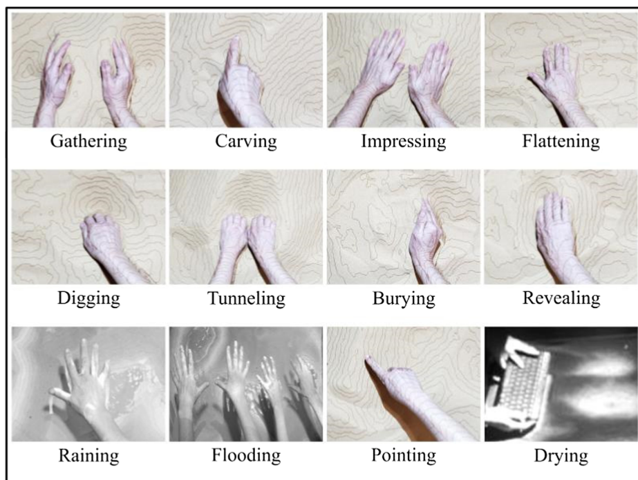
Fig. 2. Illustrated spatial actions on the sand on the AR Sandbox (colors on the AR Sandbox were removed to increase clarity)
